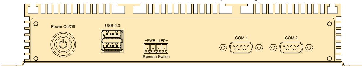
Rear Panel External I/O Mechanical Layout/Drawing
